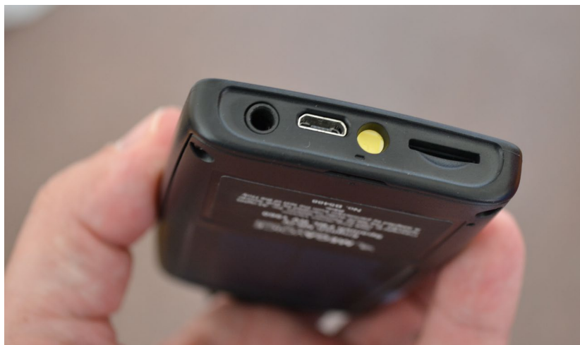
View of the bottom end of the Envoy 2 Elite: 3.5mm headphone socket, microUSB charging port, flashlight, microSD card slot
